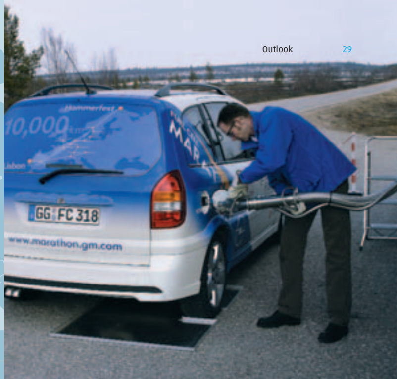
Throughout the tour, Linde supplied liquid hydrogen for fuel cell operation in the test vehicle HydroGen3.
