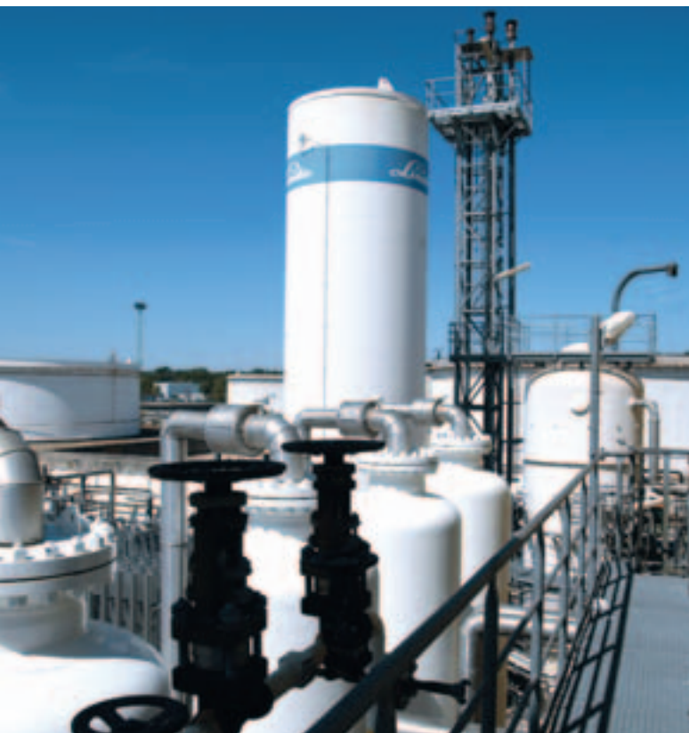
Linde constructs hydrogen liquefaction plants in various sizes. In the picture: the plant in Ingolstadt, Germany, with a capacity of 4.4 tons of LH 2 per day.
