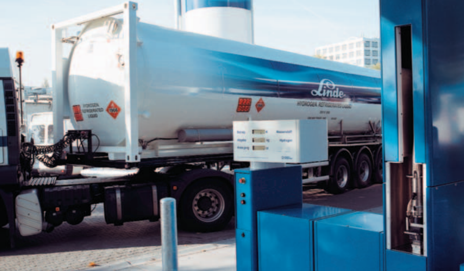
Delivery of liquid hydrogen for the LH 2 filling station.
